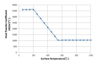
Fig.2. Heat transfer coefficient for the water cooling.
