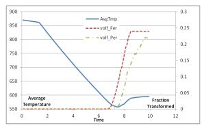
**Fig.5.** Predicted temperature and phase evolution of medium carbon steel.
