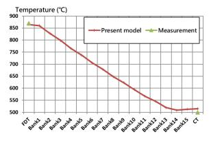
Fig.6. Predicted temperature at strip tail end.
