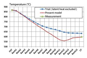
Fig.4. Predicted temperature at strip head end.
