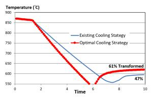
Fig.7. Optimal cooling strategy for medium carbon steel.
